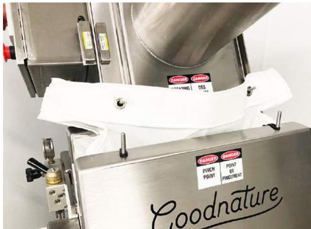
**Fig 3.1:** Press bag in grinding position
