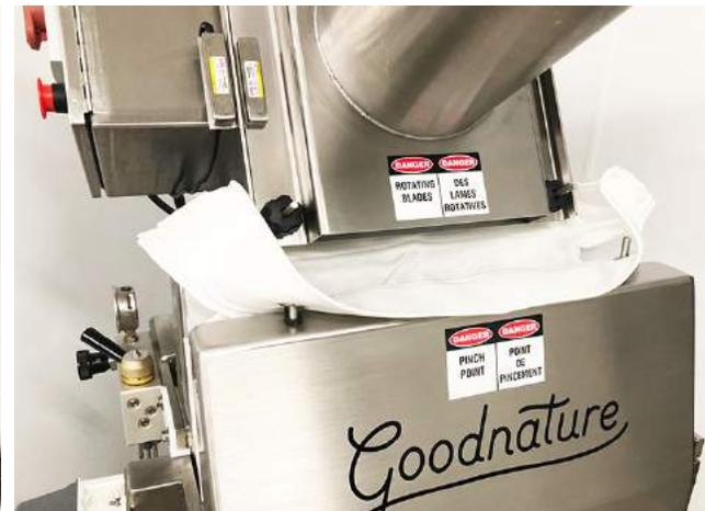
**Fig 3.2:** Press bag in pressing position
