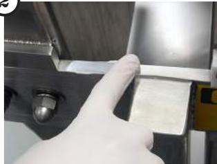
Apply food grade grease to the top rail of the X-1 allowing the shims to glide along the press with minimal resistance.
