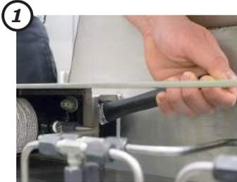
**1** Tighten large hex nuts that are at the end of the hydraulic arms. This requires a 1 1/2" box wrench which is available from Goodnature.
