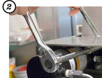
**2** Tighten the bolts and nuts that attach the hydraulic arms to the rear of the X-1 press. This requires a 9/16" wrench and a 9/16" socket wrench to tighten from both sides.
