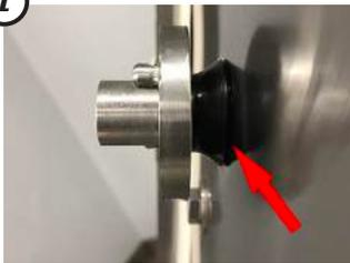
Check the black rubber shaft seal pictured at left. Lubricate with food grade grease if needed. If the seal is sitting tight against the hopper support plate, use a flat object like a screw driver to move the seal away to create space. If the seal becomes cracked or breaks over time, replace the seal.
