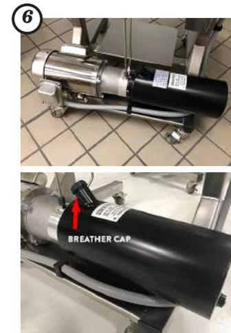
**6** Check the oil level of the hydraulic reservoir with the press fully open. Tip: Remove the breather cap and dip in a rolled up piece of paper towel. The level should be 1" - 2" (25 - 50 mm) from the top. If a drop in oil level is noticed, check the system for leaks. If oil is needed, replace with oil as detailed on the following page. Ensure the breather cap is always on during operation and cleaning. A cracked or damaged cap should be replaced immediately.
