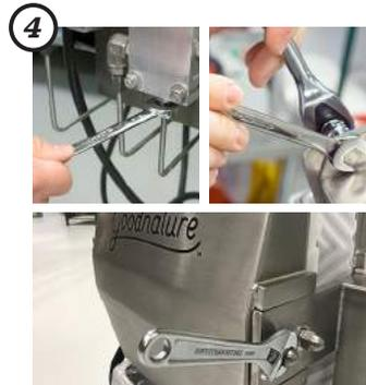
**4** Tighten all bolts, nuts, and screws visible on the machine. Do not over tighten but use wrenches to ensure they will not come loose during operation.
