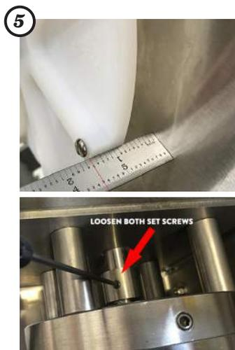
**5** Check to ensure the grinder backing disc spacing is correct. The correct spacing allows the produce to flush from the grinder area to the bag more freely and put less stress on the grinder motor and components. The spacing should be 1.5" (38mm) from face of grinder backing disc to the back of grinder area as shown. If the spacing is incorrect, loosen the set screws and adjust the stub shaft. Once the correct spacing is obtained, tighten down the set screws.
