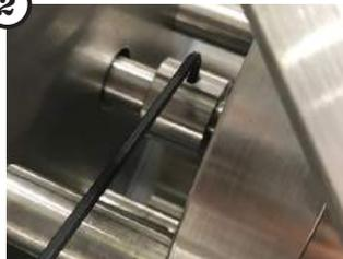
Using a 1/8" allen wrench, tighten the set screws on the drive shaft between motor and grinder plate. This will help keep the drive shaft in place and give the shaft seal room to operate.
